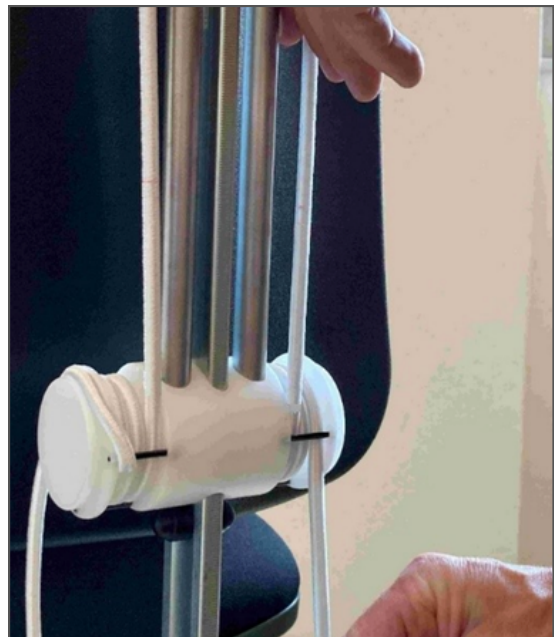
Image 40. Slide elastic until bottle touches work surface (see image 39), then lock in groove.
