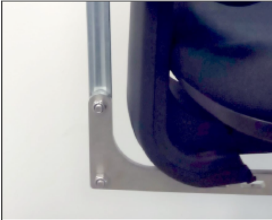
Image 12. Fix the seat bar to the vertical end of the bracket using 2 M10x30 screws and nuts.
