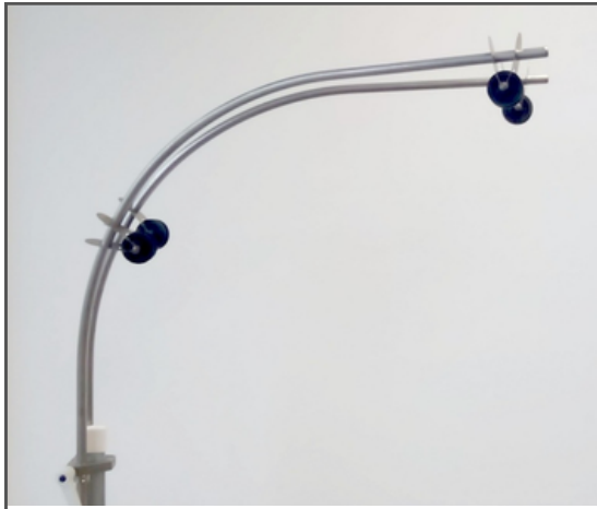
Image 22. Pinch pulleys and slide them approximately into position.
