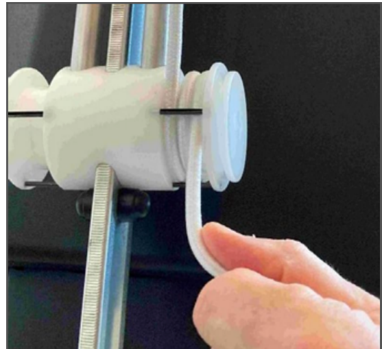
Image 31. Make 2 full turns (do NOT pass again through lower pin).
