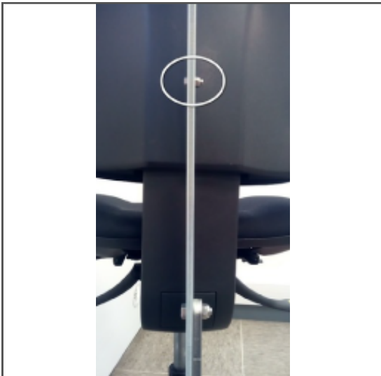
Image 14. Tighten the M6x16 screw.
