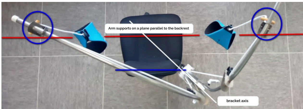
Image 11. Adjust pulley supports so that the arm supports align vertically with the elbows, in a plane parallel to the backrest.
