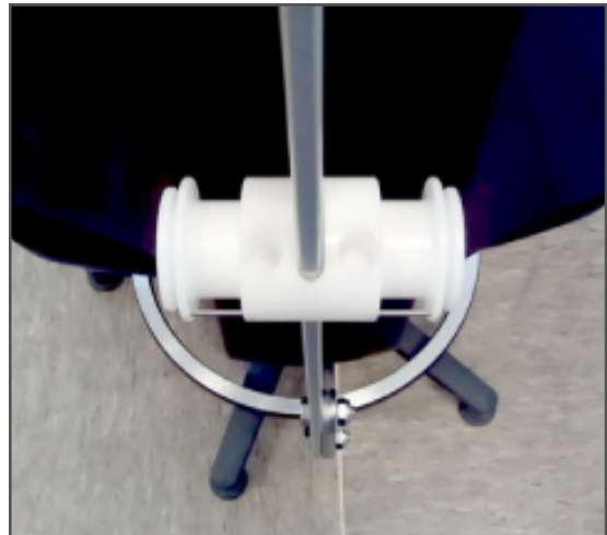
Image 15. Slide the drum with holes facing backwards.
