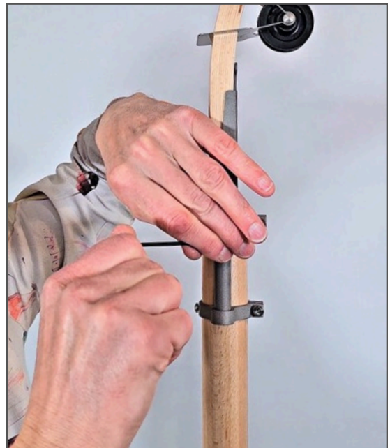
Image 22. Raise the safety ring and tighten it.
