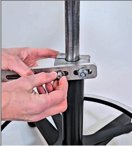
Image 9. Add the two remaining washers and nuts.
