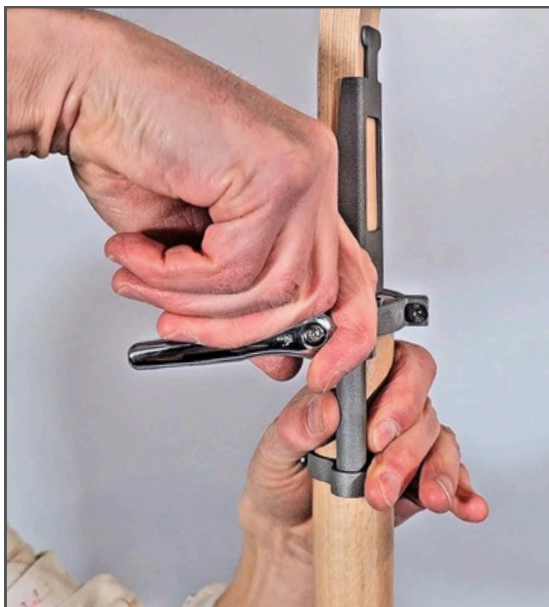
Image 23. Screw in the handles. They are indexable.
