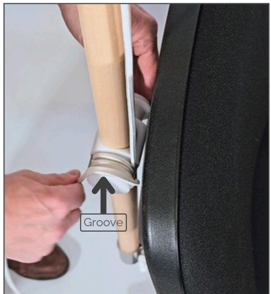
Image 32. ... lock the elastic into the drum groove.
