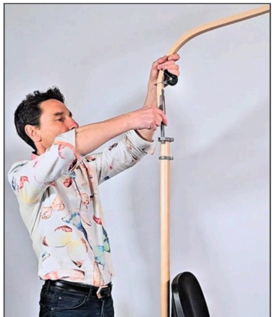
Image 20. ... then insert the assembly into the bearings.
