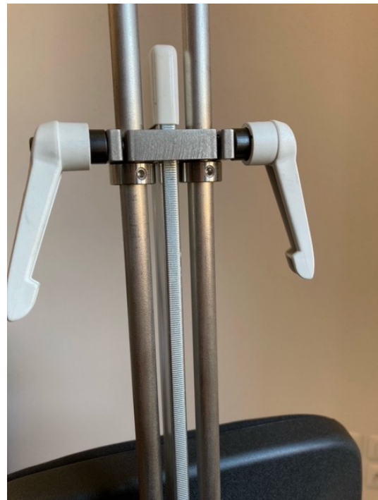
Image 25 : Slide the rings up against the collar and tighten them. These safety rings prevent the bows from rising and coming out of the holes in the drum in case of mishandling. The handles are indexable. Once locked, it is possible to orient them by pulling on them.
