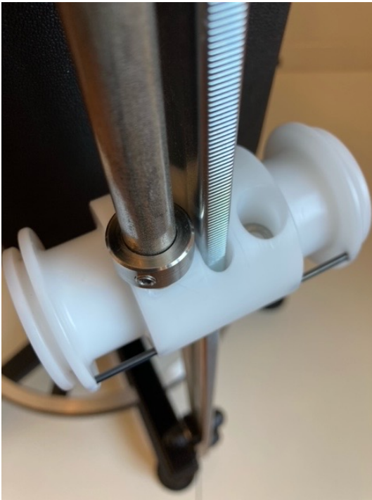
Image 22 : Do not tighten the ring for now.
