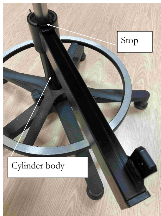
Image 11 : Lower the interface until its stopper contacts the cylinder body. The slot in the plastic ring and the slot in the interface should be opposite each other.
