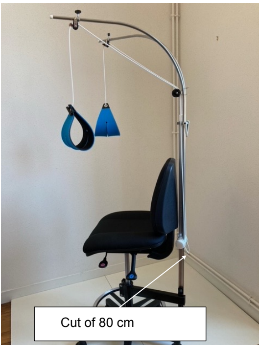
Image 40 : Optionally, cut 80 cm from the trailing part of the elastic and burn the end to prevent fraying. Be careful to ensure that the heat generated poses no danger.
