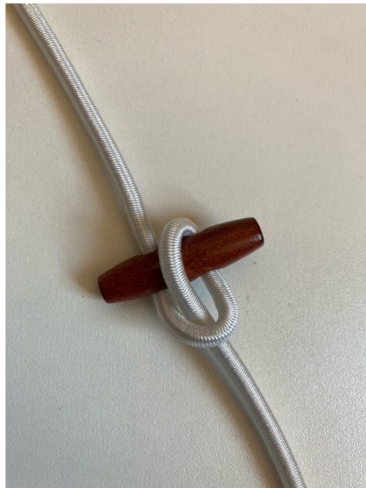
Image 30 : Assembly of the barrel button on the elastics. For this ...
