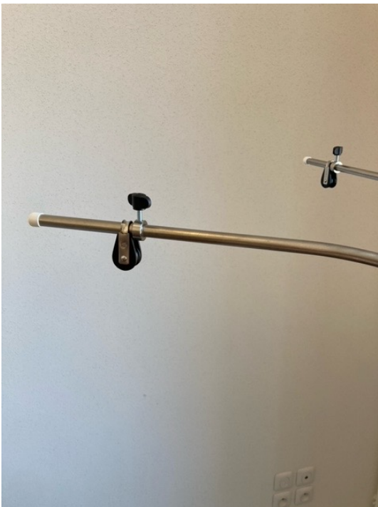
Image 29 : ... then slide the pulleys and place the two small white caps.
