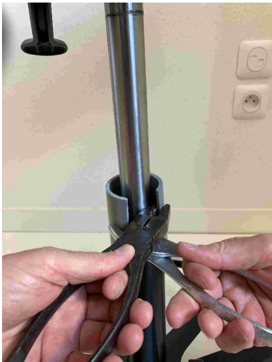
Image 8 : ... spread the ring by hand (or with pliers) to fit it over ...
