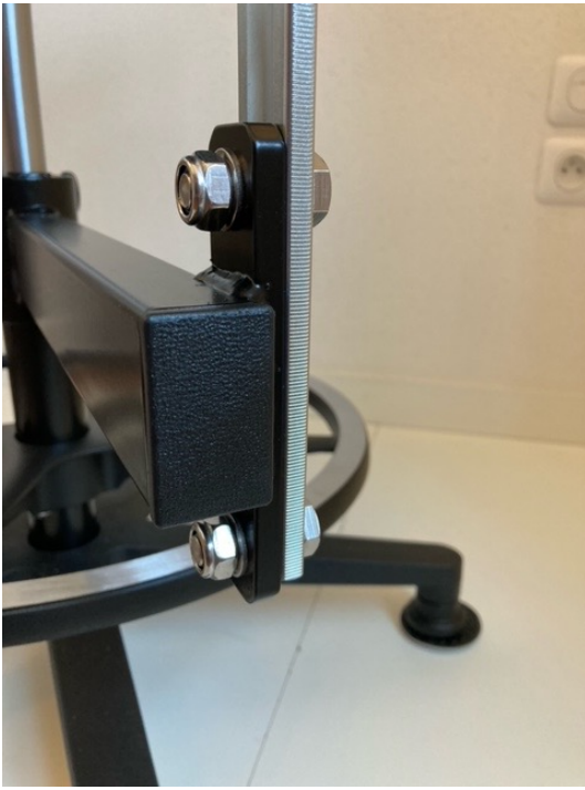
Image 14 : Assemble the clamping bar using the two large bolts.
